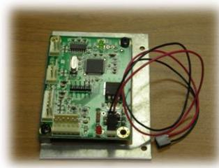
Install the controller PCBA into the base of the printer. To do this, remove the bracket shown in the picture by unscrewing the 2 screws holding it in place. Then place the controller PCBA in the printer as shown and screw it in the base of the printer using the same screws from the bracket that was removed.
