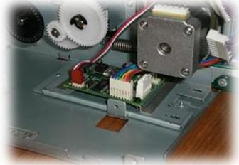
Connect the connector from the 2 Pin (Power) on the controller PCBA to the printer's power supply directly (input voltage source) as shown below.
