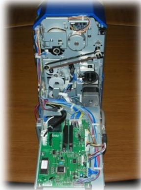
Disconnect the sensor from the wire leading to the main board and remove the emitter from the laminator.
