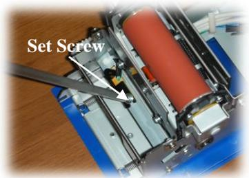
Then detach the cable and remove from the assembly. Install the new receiver in the reverse order in which the detective receiver was removed.
