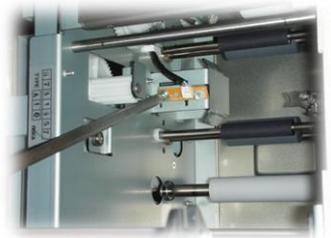
Pull the main board bracket down to access the emitter on the back side of the laminator by removing the screws shown below.
