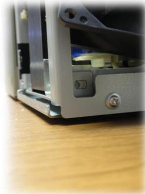
Next, attach the fan back to the frame and re-assemble the heat roller.
