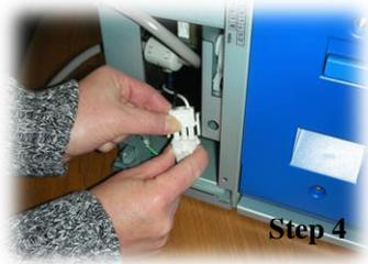
Once the transformer is in place and connected, secure it with the four screws to the frame of the heat roller.
