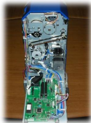
Remove the power cable by disconnecting it from the main board and the power socket.
