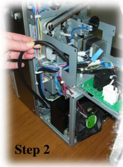
Connect the transformer to the main board & power outlet.
