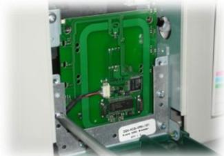
Route all loose wiring and secure to wire harnesses. Connect USB cable to host computer to test encoder (make sure Omnikey 5321 driver is installed, otherwise the encoder will not work). If the encoder is installed in the PR5350/PR5360LE, you must flash the printer with the card positioning firmware. You can download the file (pr5350lcRwS17010.dat) form our website [www.teamnisca.com](http://www.teamnisca.com) under support.
