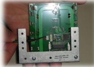
Attach the USB mini cable back onto the encoder module. Insert the encoder in the printer on an angle and secure with 2 screws.
