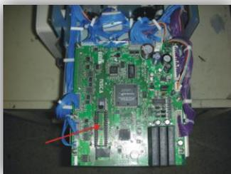
If the encoder is installed in a PR5310, then you must install the provided EPROM which holds the card positioning command in the socket of the main board.
